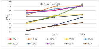
For the flexural strength test after 28 days curing, 30SGG provides the highest flexural strength closely followed by 30SGA, 15SGG, 15FA, 15SGA, all in line with the reference mixture.
