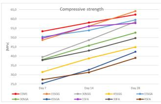
For the compressive strength test the 15SGG provided the highest results after 28 days, followed by the reference mixture and 15SGA while the 15FA is sloping more out after day 14.
